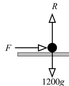
The friction  $F$  causes deceleration  $a$  which is given by Newton's Second Law,  $F = ma$
