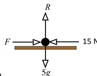
Therefore the maximum possible friction is  $F = \mu R = 0.4 \times 5g = 19.6 \text{ N}$
